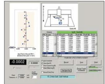
**Machine Tool Geometry — Data Taking Screen.**
