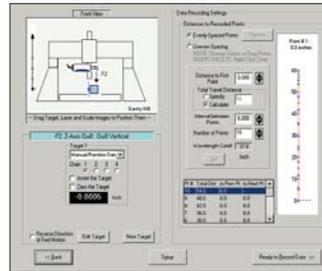
**Machine Tool Geometry — Axis Setup Screen.**
